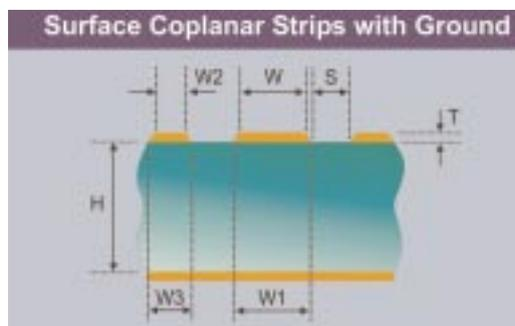
*This diagram shows just one of the many coplanar configurations .*
