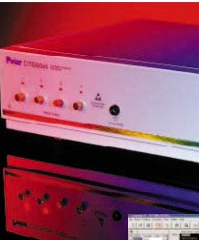
CITS uses TDR techniques to measure controlled impedances and it automatically reports when a measurement is outside the specified tolerance. It automatically processes the data to produce a simple display of impedance versus distance.
