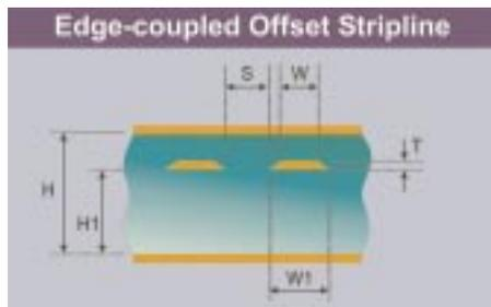
This differential configuration has two traces that are separated by laminate and sandwiched between two planes. Although the diagram shows the traces offset, the manufacturing objective is to have the traces with no offset, i.e. one should be directly above the other. Typically, this configuration is difficult to fabricate.
